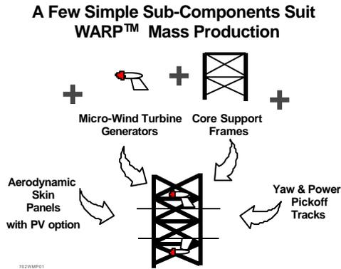
**Figure 3. WARP is Readily Volume Produced**
