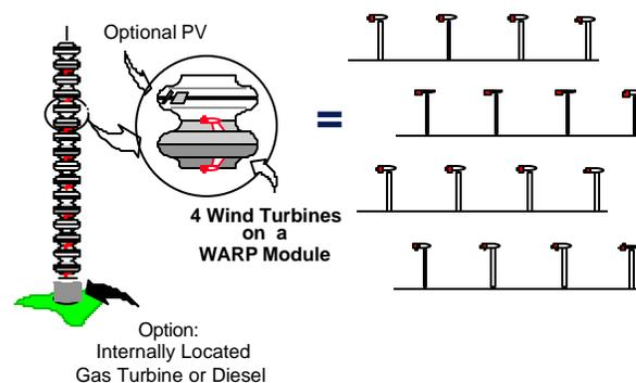
**Fig. 1 WARP Wind Power System Performance**
