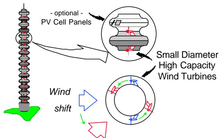
**Fig. 1a. WARP Modules Amplify Wind to 80% & Yaw into Wind**
