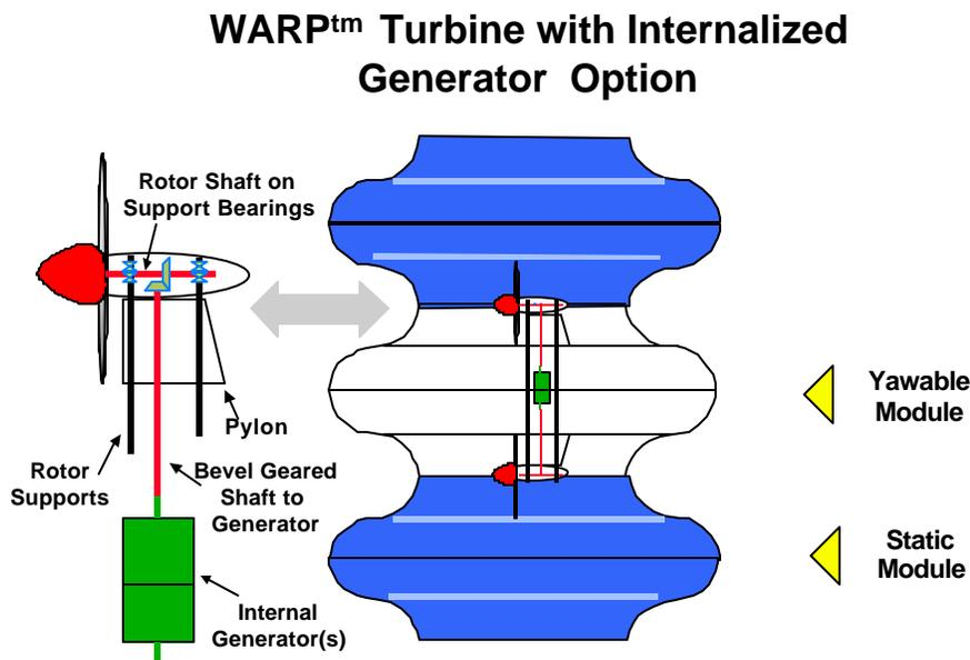
Fig. 1c Internal WARP Generators Can Provide Added Optimization, Access & Cost Benefits
