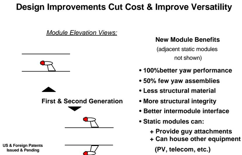
**Figure 4. WARP Design Improvements Cut Cost & Enhance Performance Further**
