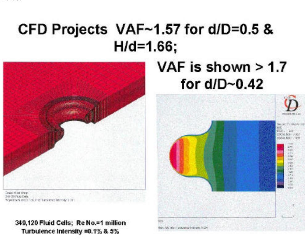
**Figure 5. CFD Analyses Show WARP Modules Can Amplify Wind Speed over 1.7 Times Free Wind**
