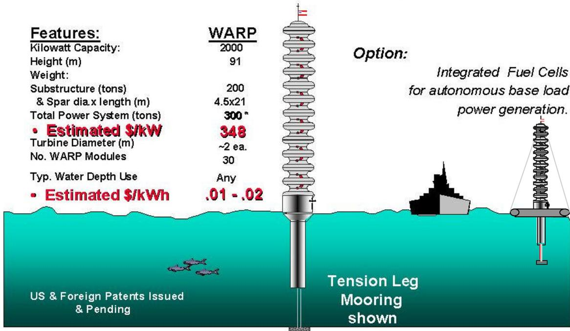
**Figure 8. A Spar-WARP Power System Can Be Flexibly Deployed
