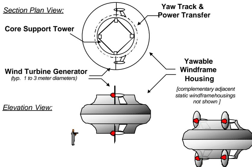
**Fig. 2 WARP Modules Can Amplify Free Wind 80% & Have Multi-Tasking Features & Benefits**
